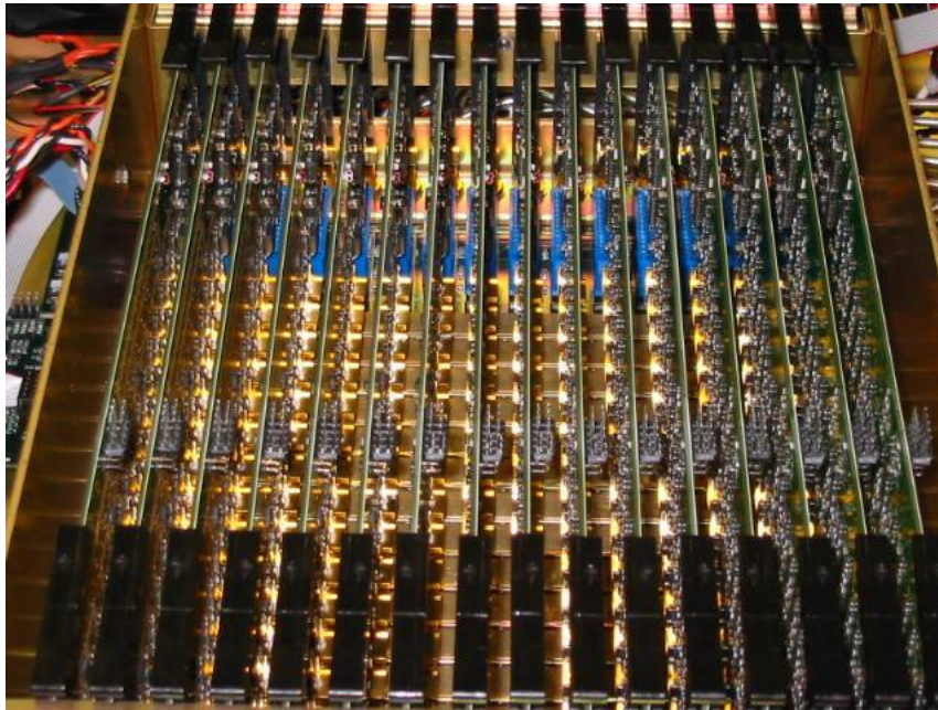
Figure 4-2 : 16x16 Switch Matrix Internal View
