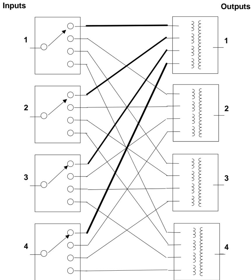
**Figure 2-3 : 4x4 Full Fan-In Non-Blocking Switch Matrix**
