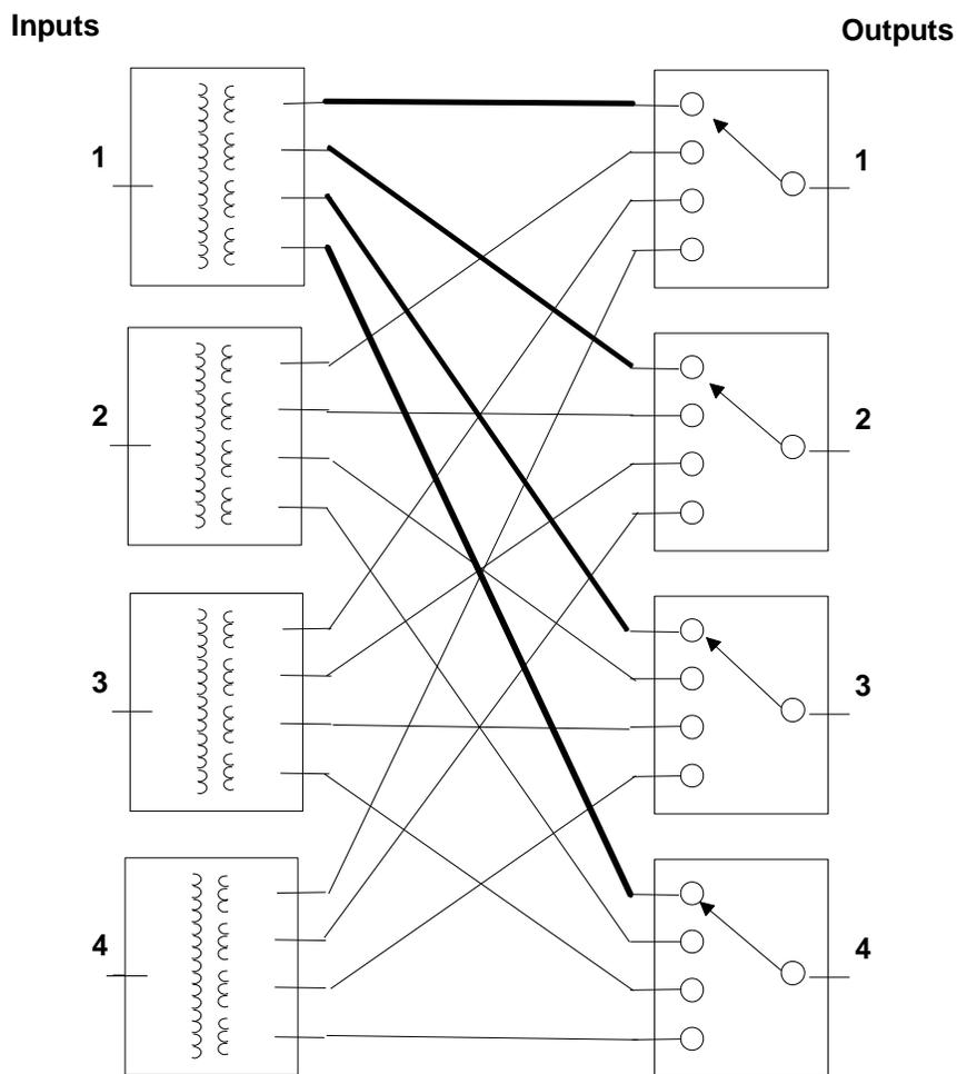
**Figure 2-2 : 4x4 Full Fan-Out Non-Blocking Switch Matrix**
