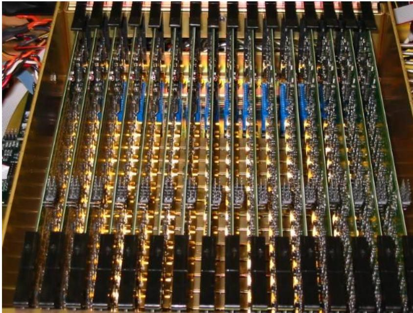
**Figure 4-2 : 16x16 Switch Matrix Internal View**
