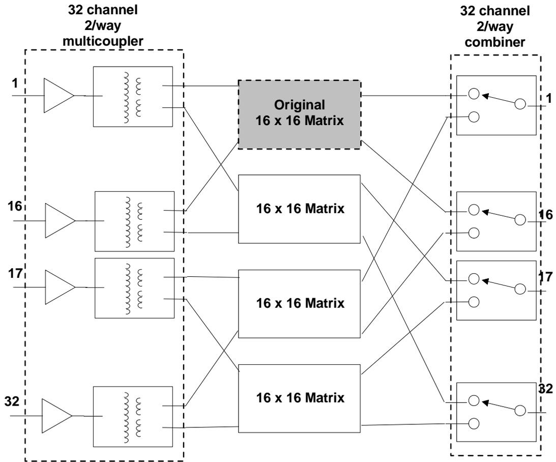
**Figure 4-3 : Matrix Expansion from 16x16 to 32x32**
