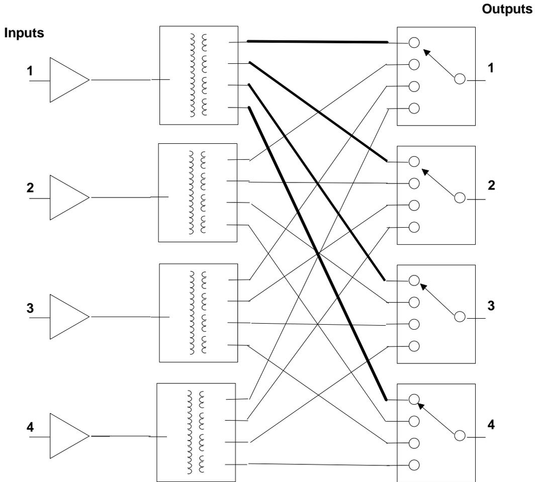
**Figure 4-1 : Amplified 4X4 Non Blocking Matrix**
