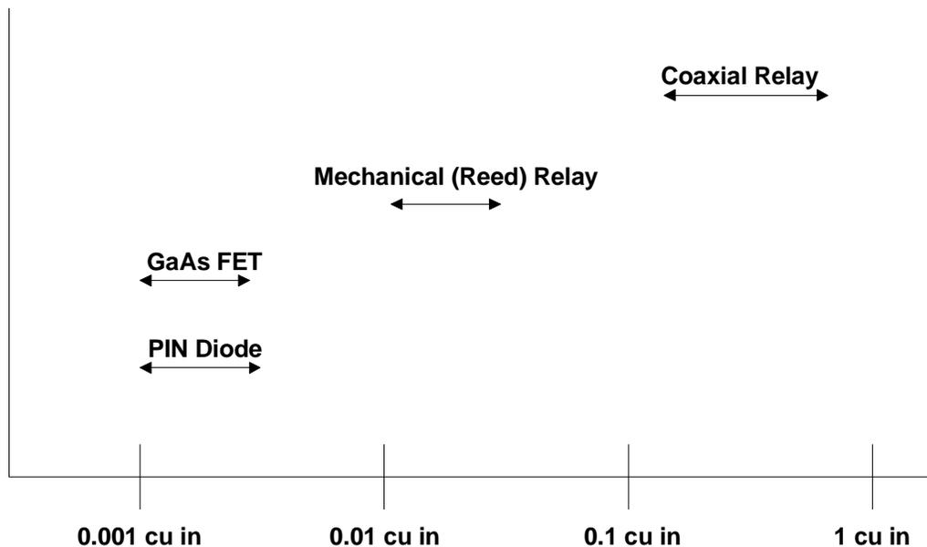
**Figure 3-6 : Switch Physical Volume per crosspoint**
